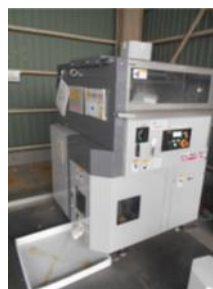
Foamed plastic melting equipment
